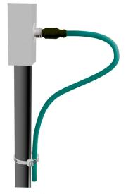
or shortening the cable's life span. The minimum bend radius is five times the cable diameter for stationary cables and 10 times for moving/flex cables. When cabling is bent beyond this pre-determined minimum bend radius, it can cause transmission failures. All pathways must maintain the minimum bend radius wherever the cable makes a bend.
